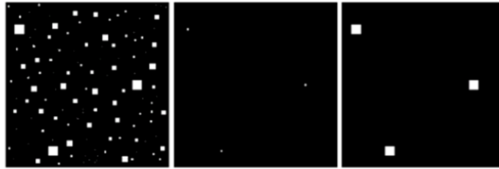
Fig.13. (left) Image of squares of size 1,3,5,7,9, and 15 pixels (middle) Erosion of left image with a square structuring element of 1's 13 pixels (right) Dilation of middle image with same structuring image
