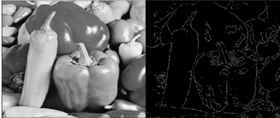
Fig.5.Examples of edge detection of the original image (left) using multi-scale wavelet (right)
