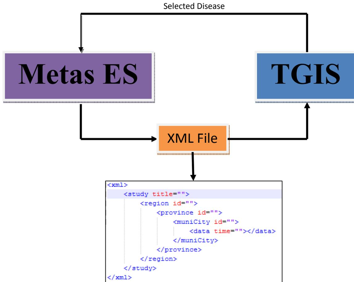
Figure 41. Simple Diagram of how the Metas ES and TGIS will communicate.
